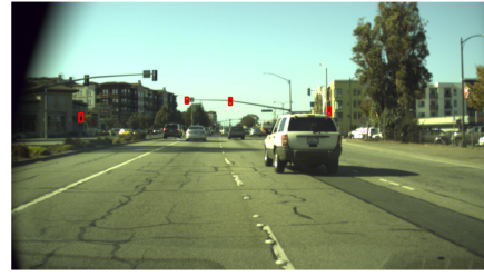
Figure 4. FasterRCNN model successfully detecting traffic lights in urban environment.
