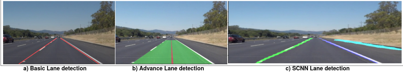
Figure 2. Three different methods for Lane detection. a) Uses Hough lines, b) Uses perspective transform and histogram, and c) Uses SCNN model
